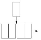
The same problem will happen if we delete an element from the middle of the array. All subsequent elements will have to be moved one space to the left to close the gap.
