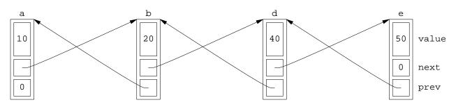
We can insert a new node c between b and d without moving any existing node.
